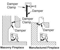
Figure 10 - Attaching Damper Clamp
